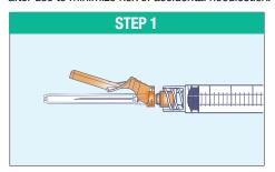
1. Carefully remove the safety needle from the package. Then securely attach the safety needle to a syringe with a push and clockwise twist motion.
